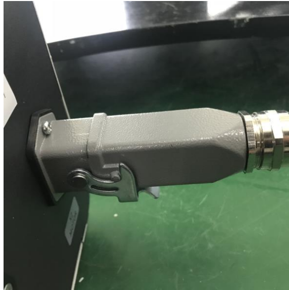
Figure 4.3 Connect controller and robot by heavy-duty cables
