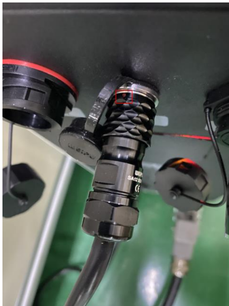
Figure 4.4 Connecting emergency stop switch
