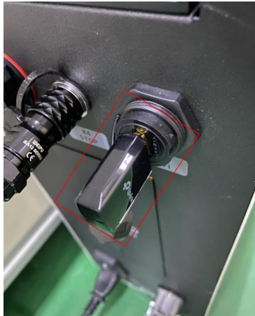
Figure 4.5 Connecting WiFi module
