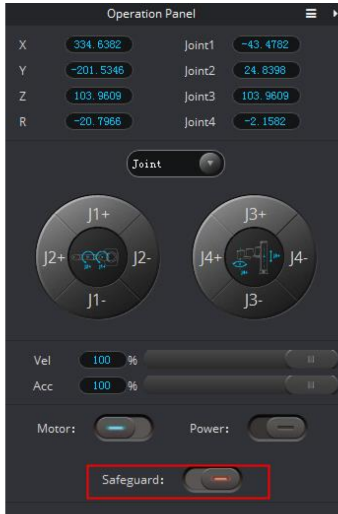
Figure 6.72 Enable safeguard stop function
