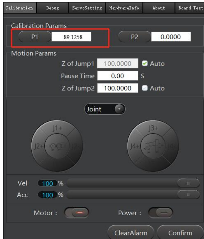
Figure 7.28 Save J2 coordinate with righty hand orientation
