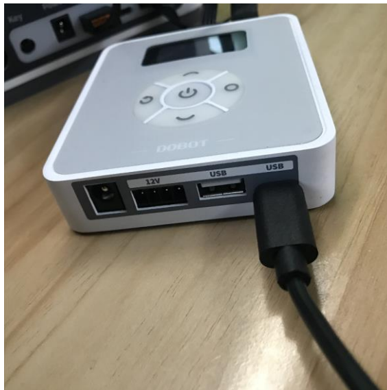
Figure 2.5 Connect Magician Lite to the electrical outlet
