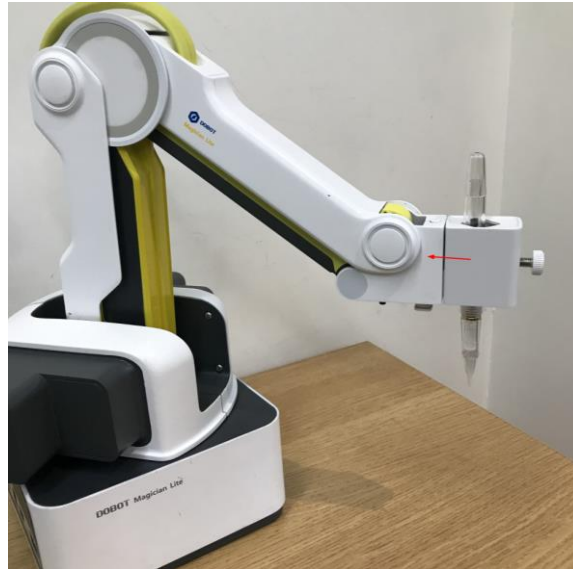
Figure 5.34 Install a writing and drawing kit
