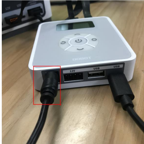
Figure 2.6 Connect power adaptor
