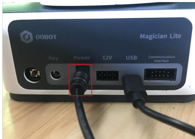
Figure 2.3 Connect Magician Lite to the electrical outlet
