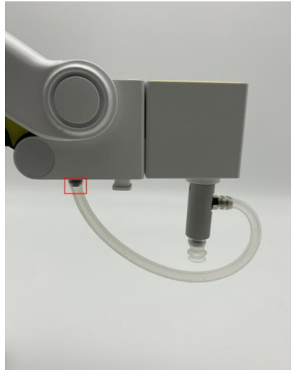
Figure 5.10 Install an air tube
