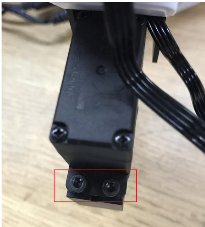
Attached figure 6 loosen the screws
