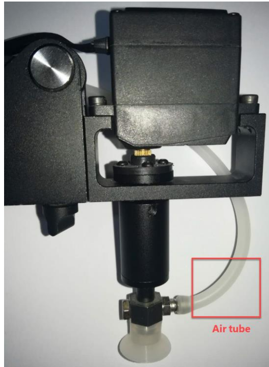
Attached figure 3 Install an air tube
