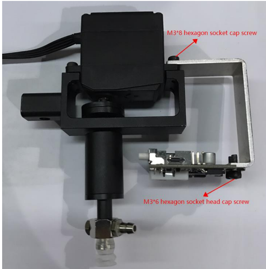
Attached figure 8 Install Pixy2 vision sensor
