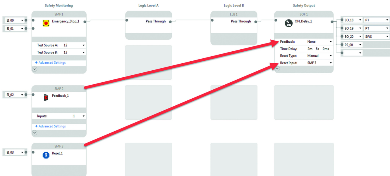
Figure 116 - ON Delay Configuration
