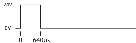
Figure 20 - N.O. Terminal Test Pulse
