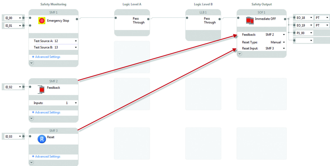
Figure 115 - Immediate OFF Configuration
