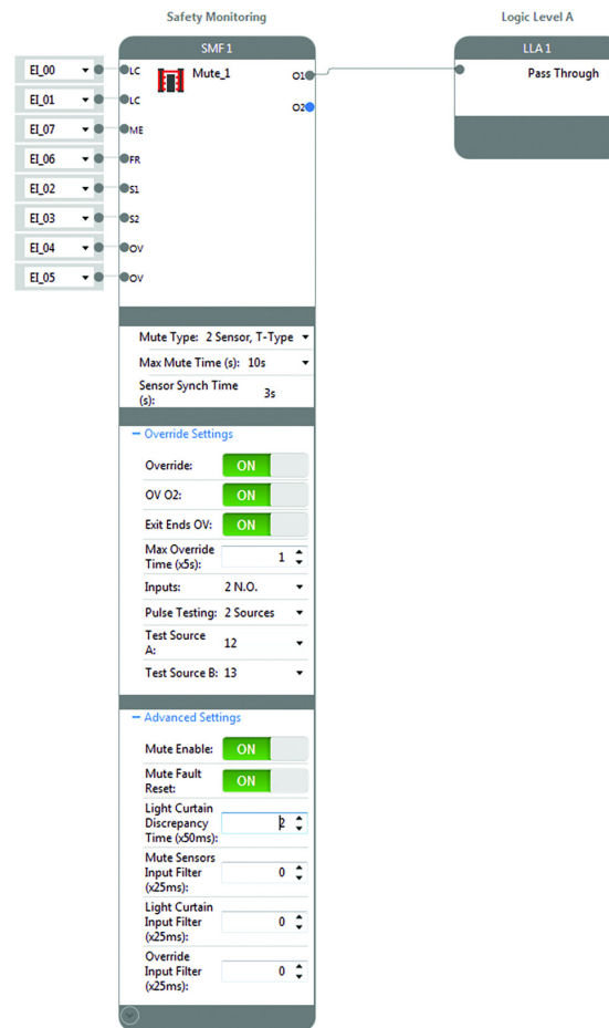
Figure 57 - Muting Function Block
