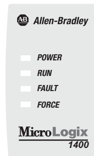
Figure 67 - Controller Status Indicator Location
