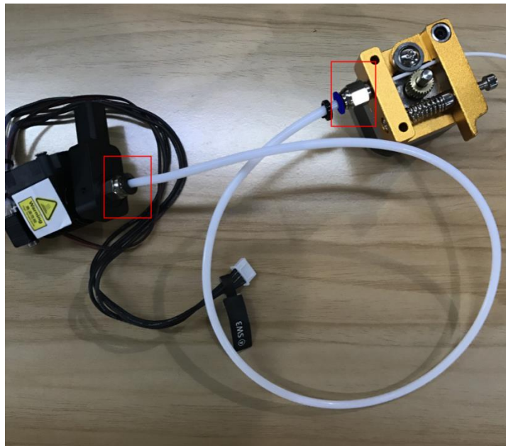
Figure 5.106 Connect extruder and hot end
