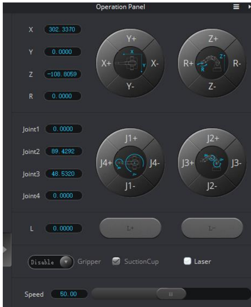
Figure 2.20 Jog the Robot Magician in the Cartesian or Joint coordinate system
