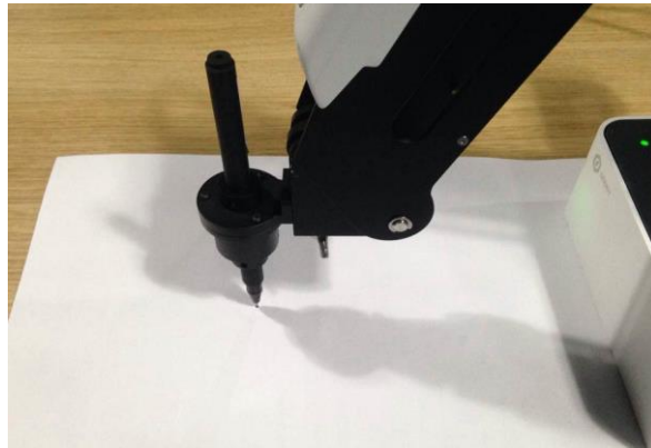
Figure 5.46 Adjust the position of the pen nib
