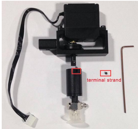
Figure 5.9 Dismantle the suction cup
