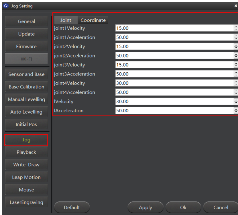
Figure 5.21 Adjust the jogging speed
