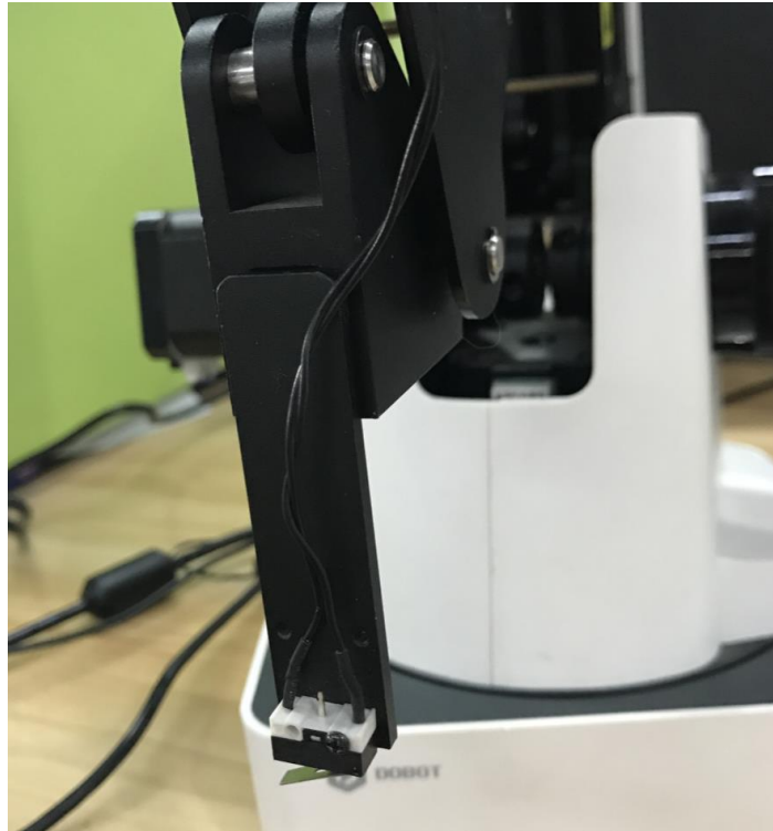
Figure 5.155 Fix auto-levelling tool
