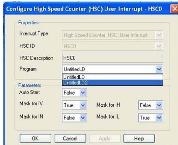
Figure 13 - Interrupt Configuration Window
