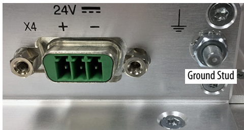
DC power input connector on the bottom of the monitor. Use the symbols for correct DC power wiring.
