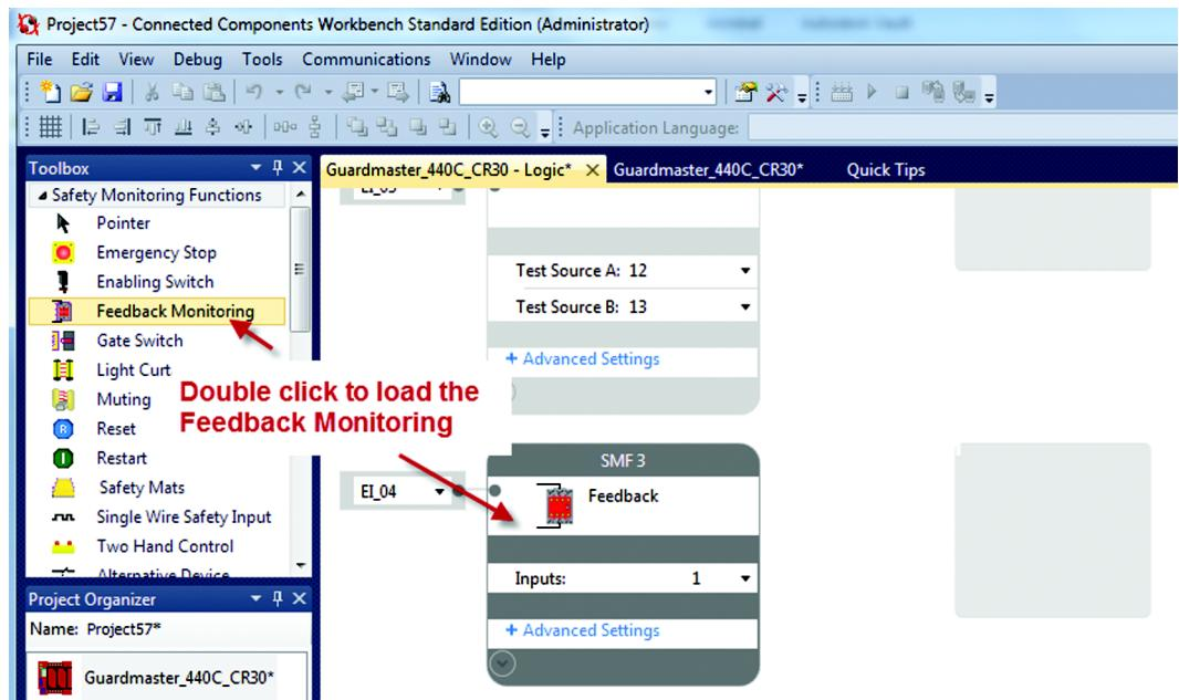
9. Modify the feedback block. Set the number of inputs to two.
