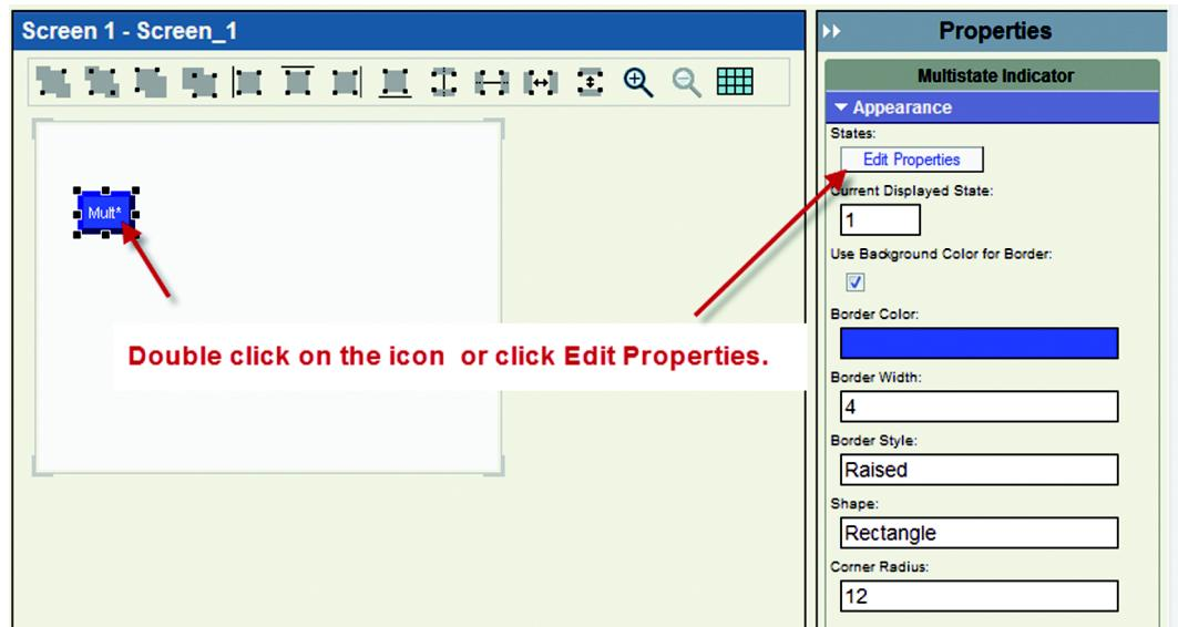
7. The multi-state indicator has a default setting of four states plus an error state.
