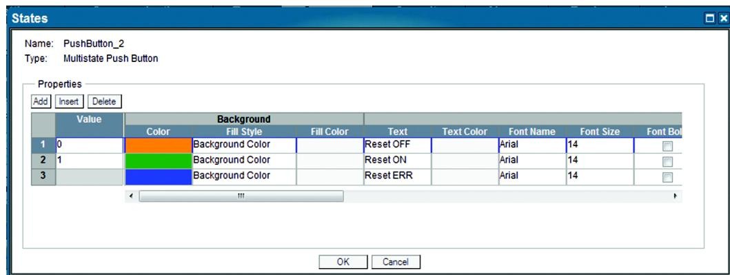
14. Stretch the reset icon and make the Write Tag connection to the reset.
