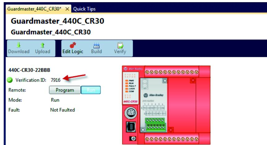
Note that the Verification ID is not saved with the CCW project file. It is saved in the CR30, so that when power is cycled, the user can upload the project from the CR30 and view the verification ID and the CR30 functions beyond the 24 hour limit.
