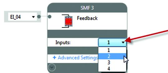
10. Assign the feedback wiring terminal. Set the Input Terminals to Plug-in 00 and 01.
