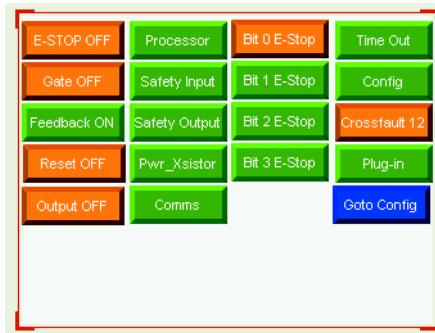
Crossfault 12 – a crossfault occurred on terminal 12, which is Input Test Pulse A.
