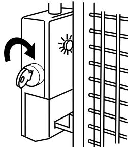
Signal is given to Atlas 5 indicating machine in safe condition & energising solenoid. Indicator also illuminates. Previously trapped key can then be rotated to release the door and hold the Atlas 5 in the unlocked mode.
