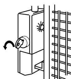
To restart the machine, the guard has to be closed & the key returned to the Atlas & rotated. Restart via normal control 'ON' button.
